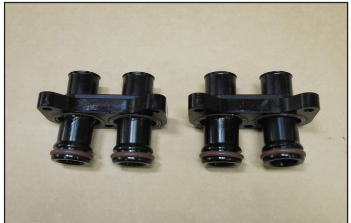
21. Reinstall the coolant manifolds with the 6 M6x20mm flange bolts that have **Loctite 242** applied and **torque them to 108 in-lbs.**
