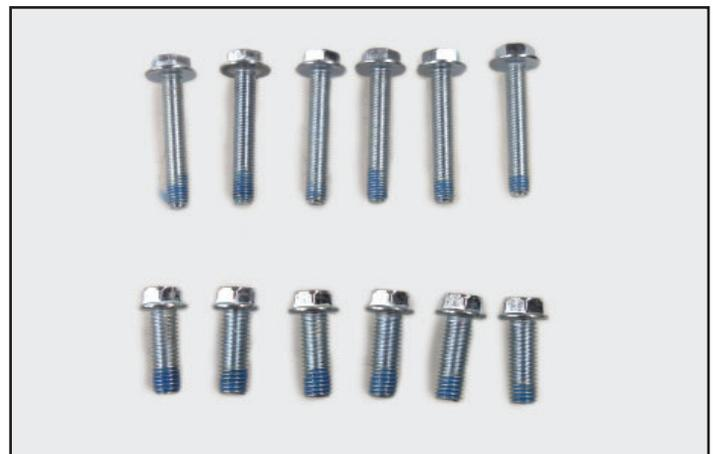
19. Reinstall the charge air coolers with the 6 M5x35mm bolts that have **Loctite 242** applied and **torque them to 70 in-lbs.**
