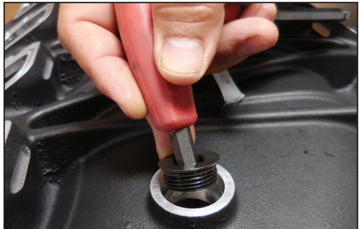
13. If you have an LT1, install the provided MAP sensor at the arrow location and secure with the supplied button head bolt shown here. **Lube the O-ring with the supplied Super Lube.** If you have an LT4 you can install your OEM TMAP in this location.
