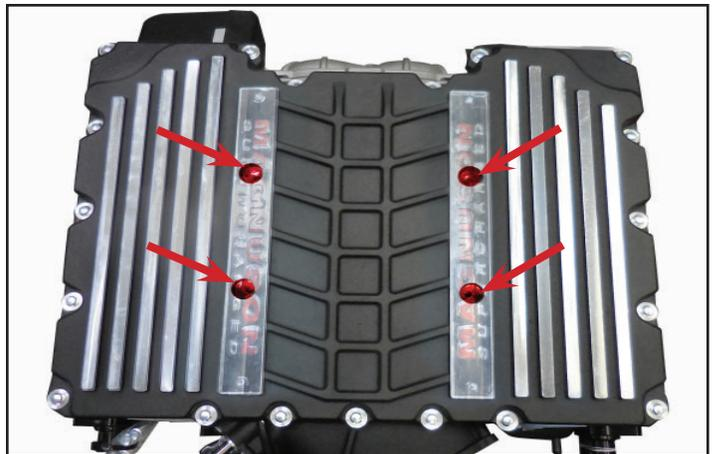
6. Remove the three M6x20mm flange head bolts (red arrows) holding the coolant manifold assembly at the front of the supercharger and pull the manifold out. Repeat this process on the other coolant manifold assembly. Note: Two boost reference locations are given at the green arrow locations.
