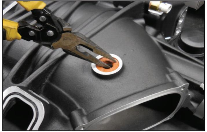
12. **For LT1 Only:** Apply a light coat of the provided Super Lube to the O-ring on the supplied threaded plug as shown below. Screw the plug into the area where the PCV seal was removed.
