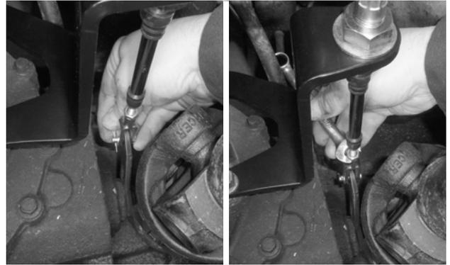
14. Attach the clevis to the range lever with the clevis pin and cotter pin, then tighten the jam nut against the clevis.
