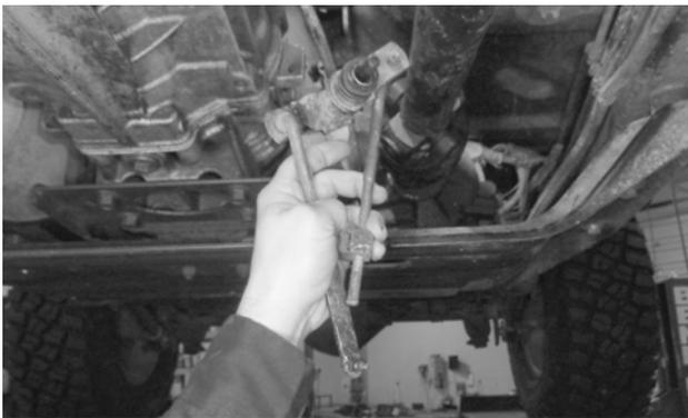
6. Remove the assembled transmission bracket, pivot shaft, and linkage rods from the vehicle.
