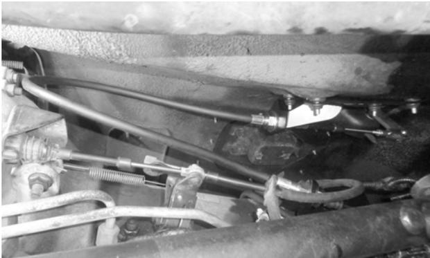
24. Verify that the cable is situated safely between the transmission and floor pan, and that it's not interfering with any moving parts.
