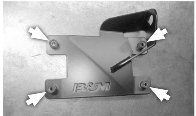
7. Push the 4 well nuts [item 7] through the back side of the floor bracket [2] as shown.
