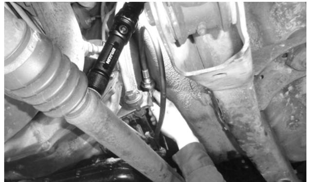
15. Install 1 washer (removed at Step 10) on the cable housing. Then route the cable forward along the transmission and back through the floor pan bracket, toward the shift lever. Avoid any obstacles (such as wiring harnesses, fluid lines, the transmission shift mechanism, etc.).
