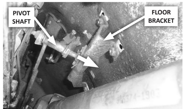
2. **Pull the floor bracket off the pivot shaft** to ease removal of the remaining mechanism.
