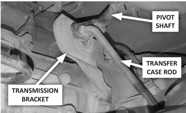
5. Remove the transmission bracket, and retain the attaching hardware.
