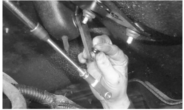
19. Install the bushing [3] in the shift lever. A dab of grease or RTV will keep it in place until the clevis is connected.
