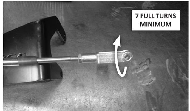
9. Install the jam nut [9] on the cable end. Then install the clevis [5] a **minimum of 7 full turns** onto the cable, and run the jam nut up against the clevis finger tight.
