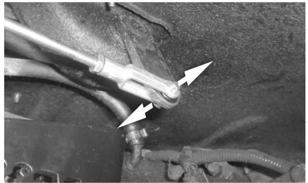
20. Adjust the cable length as required, until the clevis pin moves freely in and out of the clevis and shift lever bushing. Then finger-tighten the jam nut.
