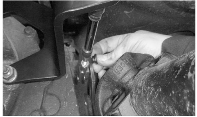
13. Install the bushing [3] in the range lever. A dab of grease or RTV will keep it in place until the clevis is connected.
