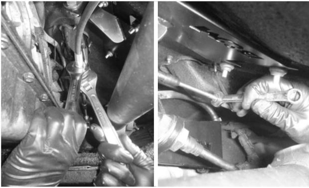
22. After verifying adjustment, tighten the large jam nuts at both brackets, and the small jam nut at the shift lever clevis.
