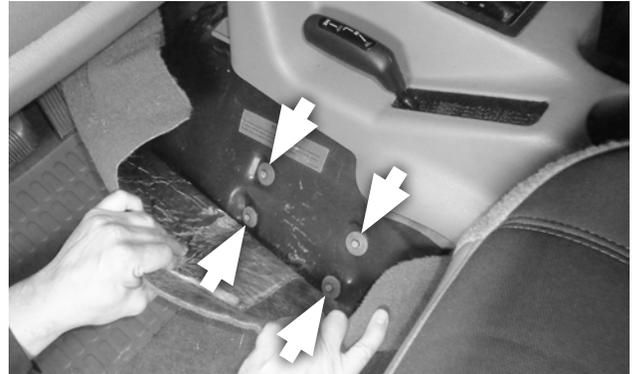
1. **Loosen the driver-side carpet sufficiently** to expose the 4 floor bracket bolts and washers, then remove them.
