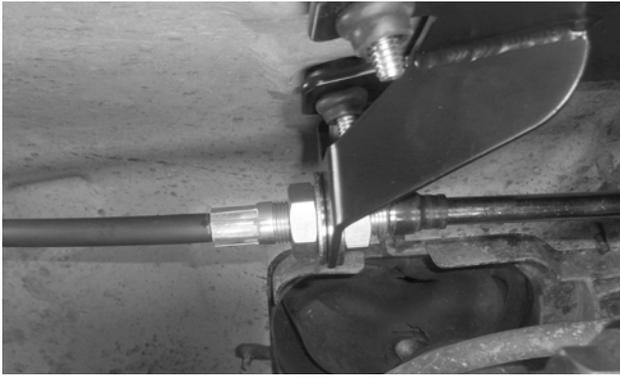
16. Install the second washer and jam nut on the cable housing. Center the bracket in the middle of the threaded section, run the nuts finger tight against it, and push the dust boot back over its joint.
