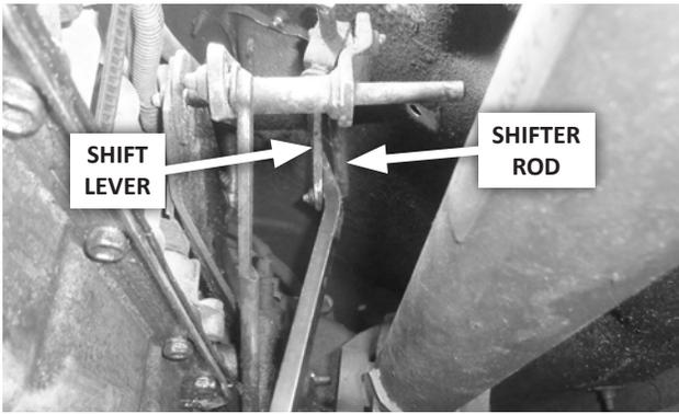
4. Pry the shifter rod end and rubber grommet out of the shift lever. If the grommet does not come out with the rod end, remove it separately.
