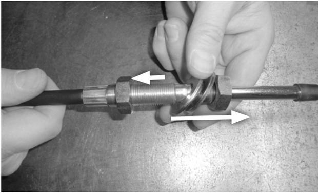
10. At the other end of the cable, remove the large jam nut and 2 washers, and set them aside. Then run the other nut down to the end of the threads.
