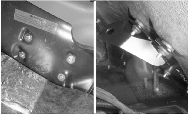
11. Install the floor bracket using 4 bolts [6] and washers [8]. Tighten the bolts until 5-6 threads protrude through the well nut.
