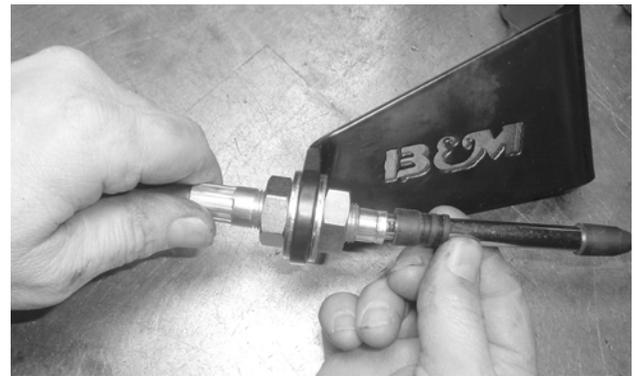
8. Assemble the cable [4] and transmission bracket [1] as shown. Pull the large dust boot off the joint to allow removal and installation of the jam nut. Situate the bracket in the middle of the threaded section, and run the nuts finger tight against it. Then push the dust boot back over its joint.
