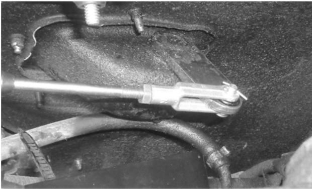
23. Install the cotter pin in the shift lever clevis pin.
