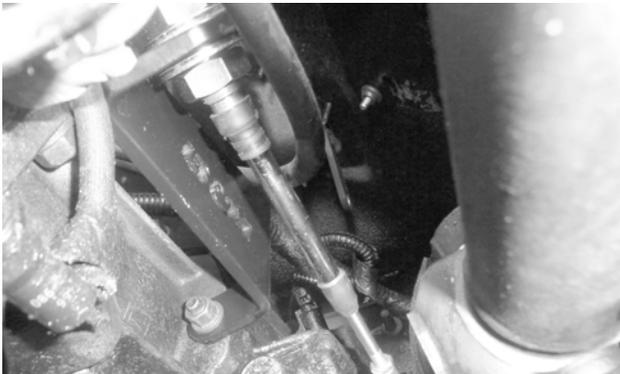
12. Install the assembled transmission bracket and cable on the transmission-transfer case split-line.
