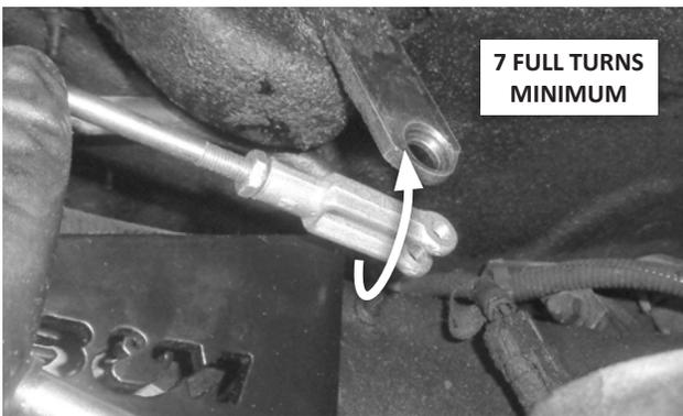
17. Install the jam nut [9], then install the clevis only [5] (no clevis pin or cotter pin), turning it a minimum of 7 full turns onto the cable.
