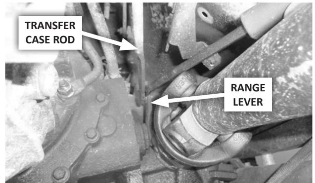
3. **Pry the transfer case rod end and rubber grommet out of the range lever.** If the grommet does not come out with the rod end, remove it separately.
