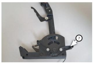
10. Remove (x2) screws from gate plate then use them to attach **switch bracket base (7)**.
