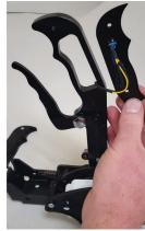
14. The shifter handle can break down to fit through narrow consoles. To do this, remove (x2) screws and driver side grip plate, (x2) screws through sub plate and passenger plate. Floss grip plate through drivers side sub plate. After fitting assembly through console, re-assemble handle.
