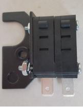
Assemble (x2) micro switches (30) to mounting bracket (28) using (x2 ea.) screws (31), split lock washers (26) and nuts (25) orienting them properly as shown.
