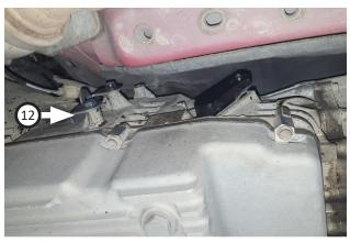
27. Fasten **cable bracket (12)** onto transmission using (x2 ea.) **flat washers (32)** and **bolts (33)**.
