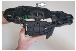
2. Remove retainer from corresponding powertrain shifter then pull pin securing components.
