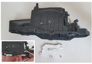
4. Press tabs and remove gear position module from shifter housing.
