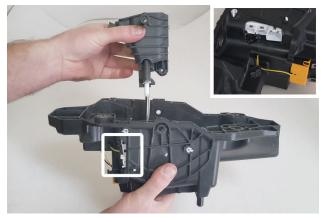
3. Remove stick assembly from housing, then disconnect all connectors (plus one inside front).
