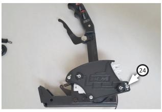
12. Fasten carrier onto shifter using (x3) screws (24). Thread in all screws only partially to allow for later bracket adjustment.
