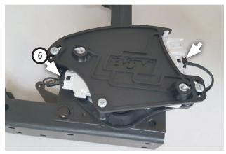
13. Connect shift buttons into gear position module rear then plug **park jump (6)** in to front.
