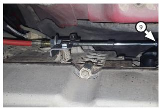
29. Thread locking washer, **nut (9)**, cable cap and remaining nut onto cable as shown.
