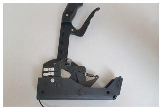
6. Attach micro switch assembly to **shifter (1)** with **slot pan screw (27)**.
