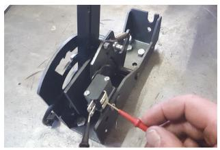
8. Using multi meter, check for continuity of each switch. Follow diagram in next step to verify.
