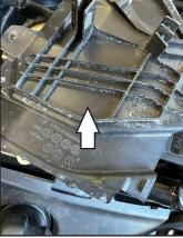
4 Secure the PC6 under the black fuel pump access panel. Double-stack the dual lock to get the PC6 off the ribs.
