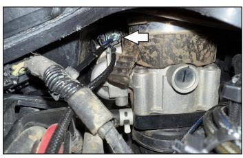
9 Attach the PC6 harness to the TPS and stock wiring harness.
