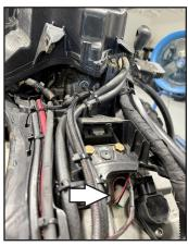
7 Route the PC6 harness along the wire loom on the left side of the vehicle.
