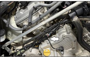
10 Unplug the fuel injector and plug the PC6 harness inline on both cylinders.
