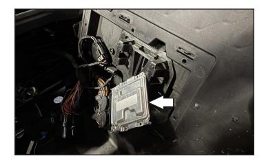
3 Remove the three small screws securing the ECU. Save these screws if you may want to reinstall the stock ECU at a later date.
