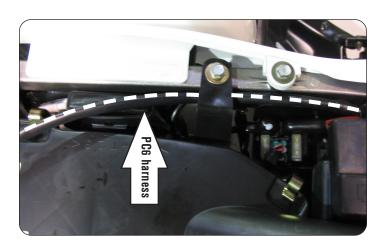
A Route the PC6 wiring harness from the rear of the quad to the throttle body going along the left hand side of the frame.
