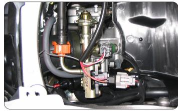
9 Unplug the Throttle Position Sensor connector from the right hand side of the throttle body.
