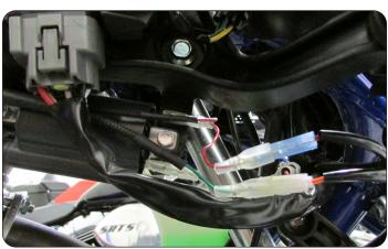
Locate the ignition coil on the right hand side. Plug the PC6 in-line of the stock wiring harness and coil.
