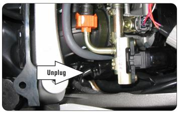
10 Connect the PC6 wiring harness in-line of the stock TPS and wiring harness.
