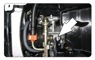
8 Plug the PC6 wiring harness in-line of the fuel injector and stock wiring harness.
