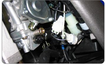
13 Plug the connectors from the PC6 in-line of the stock wiring harness and crank connector.
