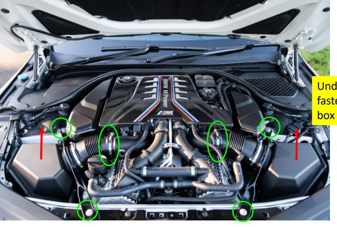
Undo the following fasteners and lift the box up as a unit.
