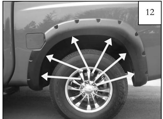
Insuring the flare is properly located on fender, apply moderate pressure to outside surface of flare, tighten all screws, beginning with the factory screw working toward the front of the fender flare.
