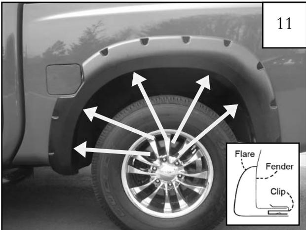
Install five Clips (CL1-0005) over fender lip, lining up the hole in Clips with the holes in flare. Start Screws (SW1-0050) in each Clip. *Do not fully tighten screws.*
