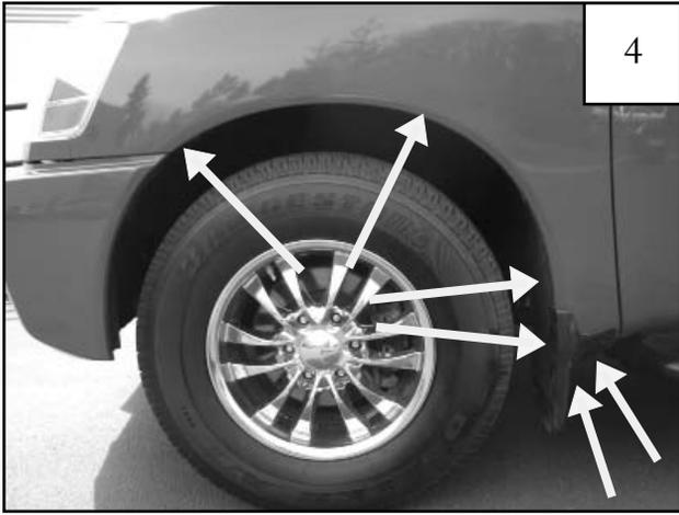
Remove factory mud flaps if installed, and one extra unpainted screw above mud flap. Also remove screw located at front of fender just above bumper. If no mud flaps were removed, remove two unpainted factory screws per side. *Save for reinstallation.*
