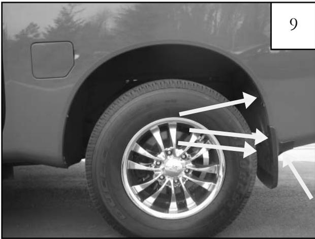
Remove factory mud flaps if installed, and one extra unpainted screw above mud flap. *Save for reinstallation.*
