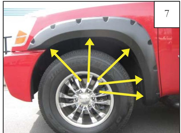
Insuring the flare is properly located on fender, apply moderate pressure to outside surface of flare, and tighten screws, beginning with the two rearward factory screws working toward the front of the fender flare.
