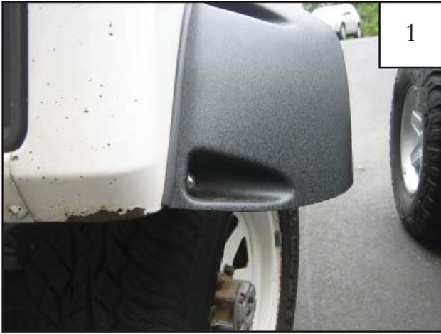
The front and rear flares are similar in shape and size. Front flares are labeled on the inside with 60015-07 and rears are 60016-07. Pictured above is the front flare.
