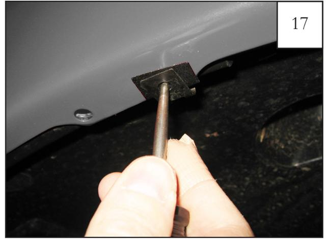
Using an awl or similar pointed tool, poke a hole through Tab (MT1-0014) using the Clip (CL1-0022) hole as a guide. Repeat Steps 15-17 for remaining (2) empty hole locations.
