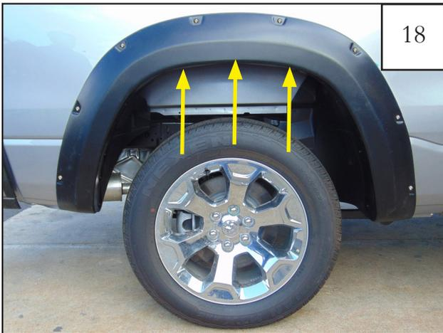
Hold flare in place and start Screw (SW1-0056) using a Phillips screwdriver in (3) locations as shown. **Do not tighten. Continue to Step 21.**
