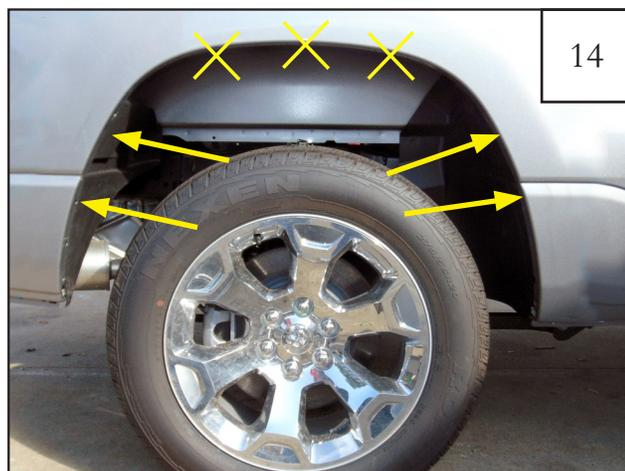
Remove (4) factory installed screws using an 8mm socket wrench. Keep screws for installation of the rear flare. X's indicate an existing factory hole that is empty.
