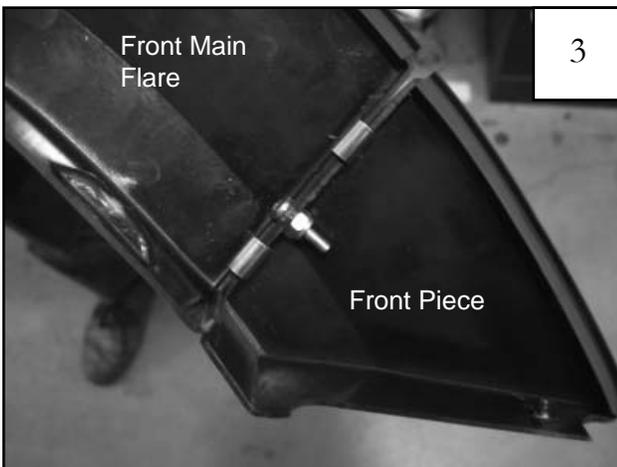
Secure pieces with two SS U-Clips (CL1-0001) to prevent rotation out of alignment after installation.
