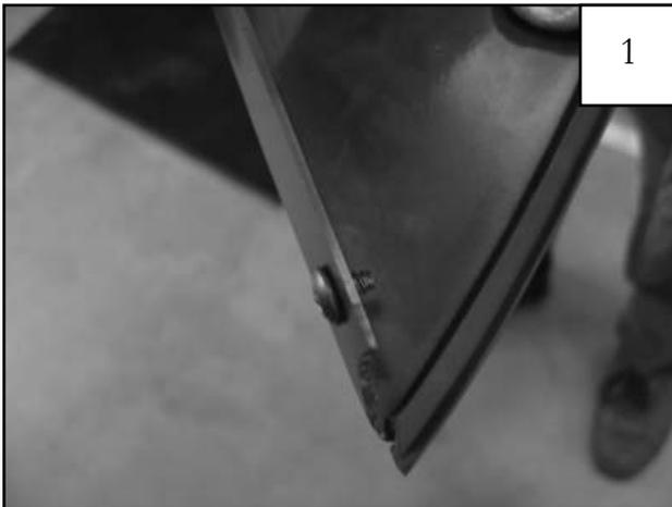
Using dimple in front piece as a guide, drill a 1/8" hole and install supplied screw (SW1-0050) through the drilled hole.
