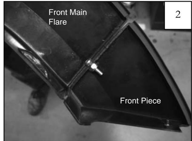
Bolt front main flare and front pieces together with supplied screw (SW1-0003) and supplied nut (NU1-0004). Use a 3/8" wrench to hold nut in place.
