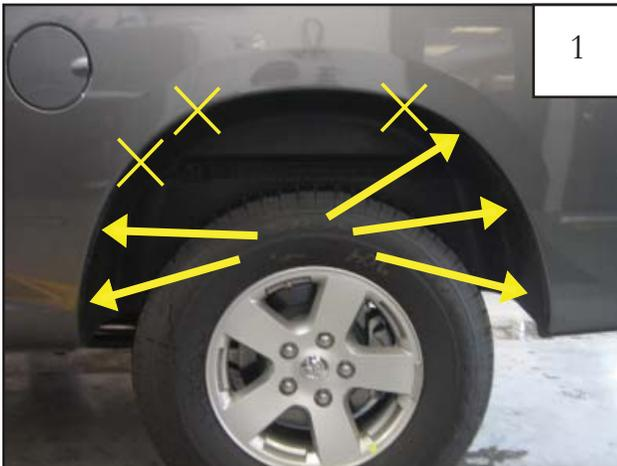
Remove these five factory installed screws using an 8 mm socket wrench. Keep screws for installation of the rear flare. X's indicate a factory screw that will not be removed.
