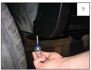
Using a Phillips screwdriver, start two supplied Screws (SW1-0049) into Clips installed in Step 8. If necessary use an awl to locate holes and adjust clips. *Note: Do not tighten. Check flare position and make sure flare fits into style line.*
