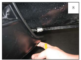
Pull back each end of flare and install assembled Clips (CL1-0008 & CL1-0010), aligning holes in clips with marks made in Step 6. The snap lock feature of the Clip should be facing outward.
