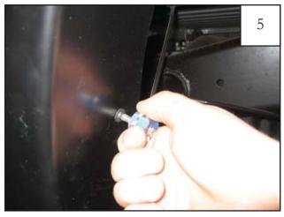
Using #2 Phillips Screwdriver, insert a supplied Truss-Head Screw (SW1-0056) through existing holes in flare and into holes in clips (4 places).
