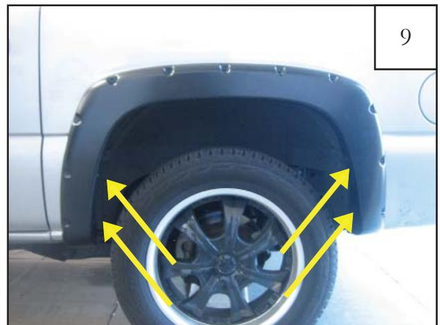
Start the remaining four Screws (SW1-0056). *Do not tighten.*
