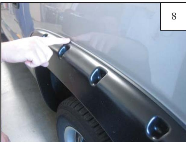
Ensure that the topmost edge of the flare is seated in the groove of the vehicle body.
