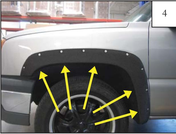
Hold front flare in place on fender and secure with supplied Fasteners (RV1-P001) through the holes drilled in the flare and into the holes in the fender body wheel well. Start at the front and work toward the rear.
