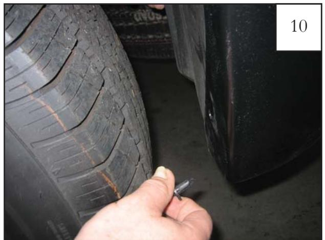
Install three supplied Plastic Push Retainers in remaining holes in flare.
