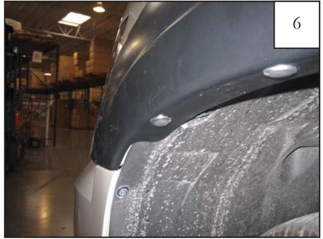
Install a supplied Plastic Push Retainer through forward hole in flare.
