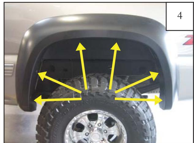
Install six tuflocks using a #2 stubby screwdriver.
