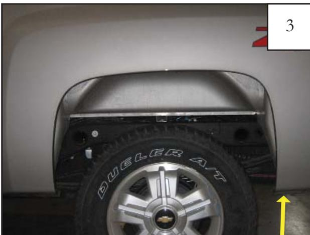
Remove one factory bolt with a 1/2" wrench.
