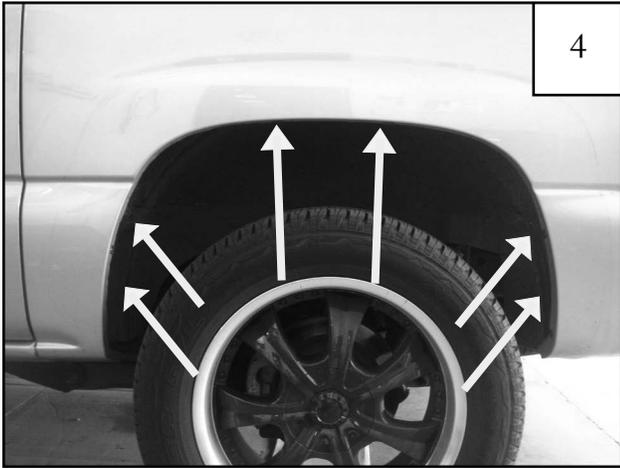
Place Clips (CL1-0022) over the six factory holes that line up with the holes in the fender flare. *NOTE: There may be extra factory holes not used for installation.*
