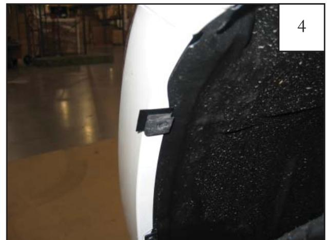
Slide a supplied "S" clip over each tab applied in step 3.
