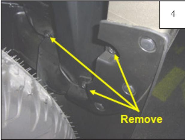
If factory mud flap is installed, remove three factory screws from the mud flap. Save screws for reinstallation.
