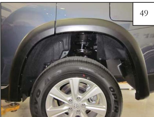
Close door and check for proper alignment between Door Piece and Rear Main Flare then apply pressure at each fastening point and tighten all Door Piece screws.
