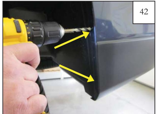
Using a 5/16" drill bit, drill two holes in wheel well lip at rear of wheel well. Use lowest dimple and third lowest dimple in wheel well lip as a guide. Install Clip (CL1-0022) at each of the drilled locations.
