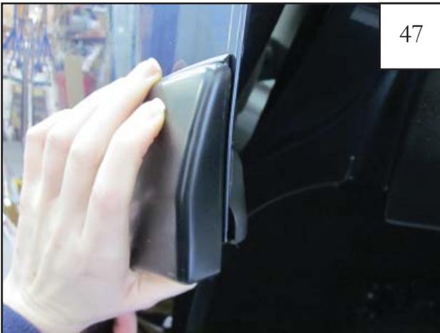
Position Outer Door Piece over Inner Door Piece, checking for proper alignment of top of Outer Door Piece with the edge of the door.
