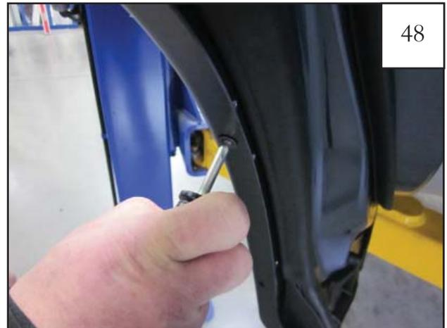
Using a #2 Phillips Screwdriver, start supplied Screw (SW1-0056) through Outer Door Piece and into clips installed on Inner Door Piece. Three locations.
