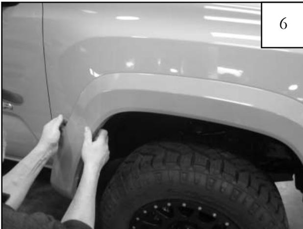
Remove flare by pulling part away from side of vehicle
