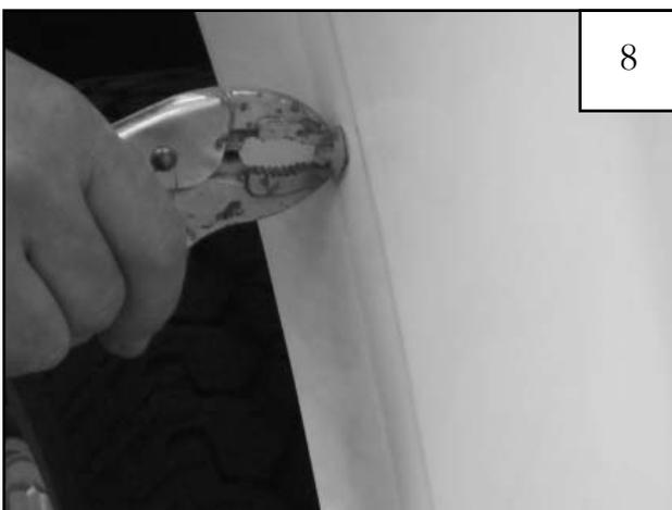
Remove one clip from front using vise grips, pulling with a rocking motion. See step 9.
