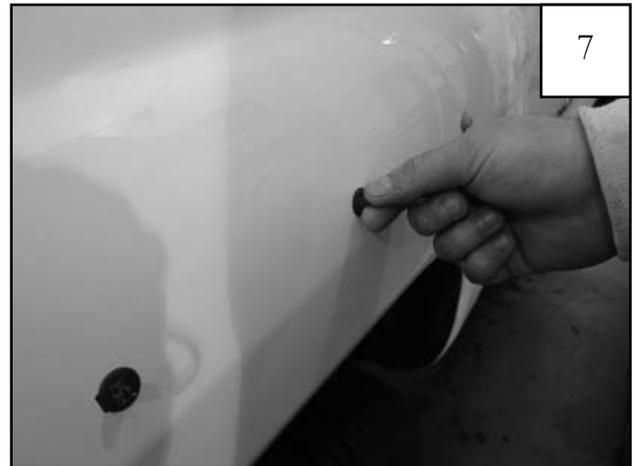
Using a clockwise twisting motion, remove eight factory plastic clips from fender. See step 9.
