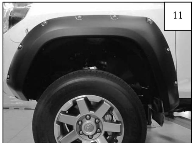
Installation Complete. Repeat process for other side of vehicle.
