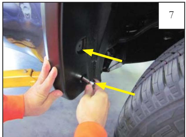
Start two supplied 20mm Hex Screws (SW1-0036) through the rearward most holes of flare and into the factory hole in fender.
