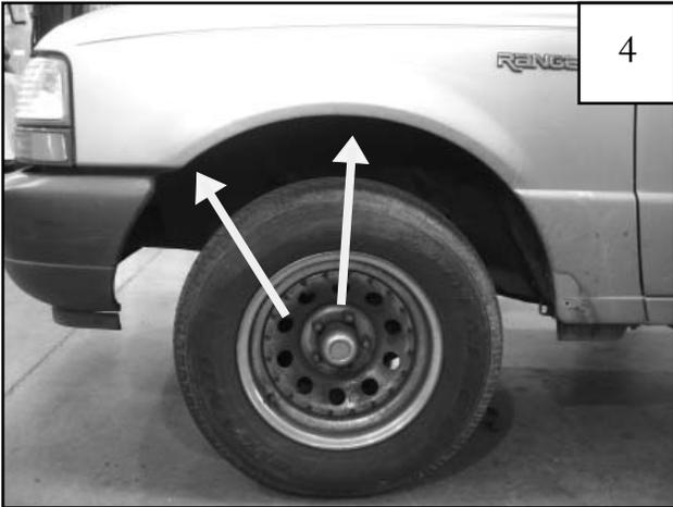
Remove factory flare, mud flap, or rock guard and clean wheel well opening. Remove two fender inner liner factory screws with a 7/32" socket wrench. Save screws for reinstallation.
