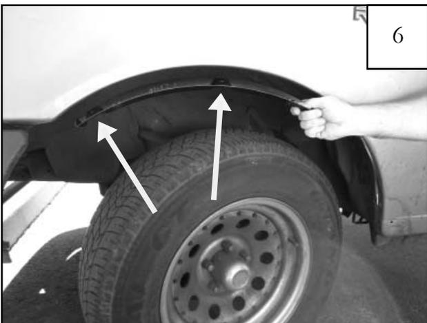
Install inner piece by hand starting factory screws, saved from Step 4, into factory holes.
