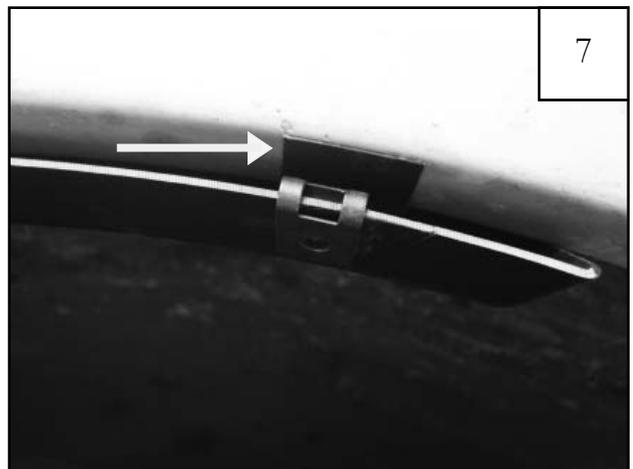
Install Tab (MT1-0002) on sheet metal between inner piece and wheel well at two inner piece Clip (CL1-0022) locations. Tighten factory screws.
