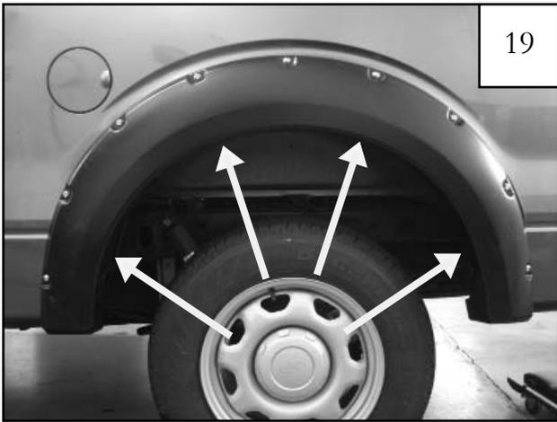
Hold flare to vehicle and start Screw (SW1-0058) through the two topmost holes in wheel well. Then start Screws through remaining holes in flare. Tighten all Screws.
