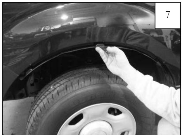
Line up the holes in the inner piece with the two uppermost factory holes and the installed clip (CL1-0011). *NOTE: Driver's side inner piece is marked with an "L" and passenger's side inner piece is marked with an "R".*
