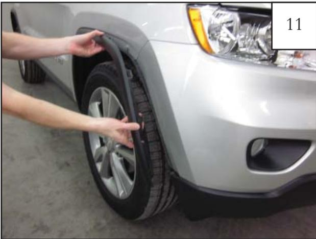
Working your way along the top and down the back side of wheel well, remove the factory flare completely from vehicle.
