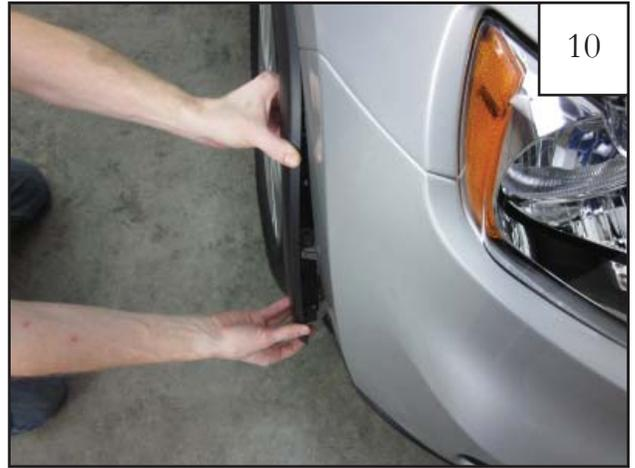
Starting at the front end of the factory flare, firmly grip part and pull to remove from vehicle. *Note: You will hear popping sounds as the factory fasteners release from vehicle. This is normal.*
