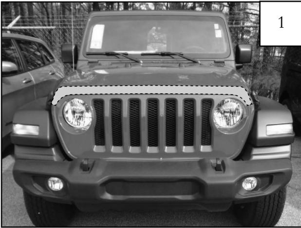
Prior to installation, wash the hood of vehicle and dry with a clean cloth. Use the alcohol pads to clean entire LEADING EDGE of hood. **NOTE: Temperature should be at least 60°F for proper tape adhesion.**
