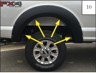
While holding flare to vehicle, start supplied screws (SW1-0058) through the four topmost mounting holes in flare and into the clips installed in Step 8.
