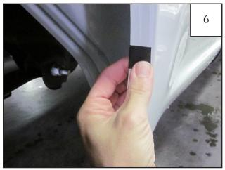
Wrap a Foam Tab (MT1-0034) around the wheel well sheet metal, centered over each of the upper four marks made in Step 5. Place a Mylar Tab (MT1-0014) at the mark made on the lower front of the wheel well.
