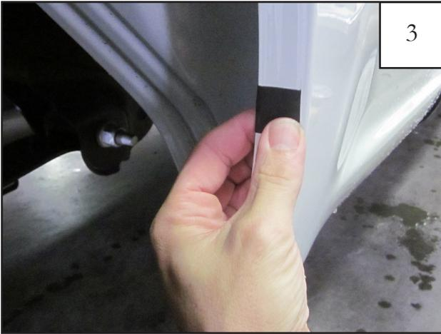
Wrap a Foam Tab (MT1-0034) around the wheel well sheet metal, centered over each of the upper four marks made in Step 2. Place a Mylar Tab (MT1-0014) at the mark made on the lower front of the wheel well.
