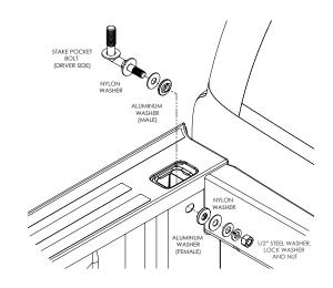
For each stake pocket bolt (driver and passenger) install nylon washer and aluminum washer over the rubberized end. Install the assembly into the stake pocket, and through the slot on the truck bed. Install the mating aluminum washer, nylon washer, 1/2" steel washer, lock washer and nut. Leave assembly finger tight at this stage.
