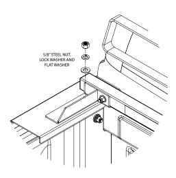
Fasten Backrack Assembly to the Stake pocket bolt as shown.
