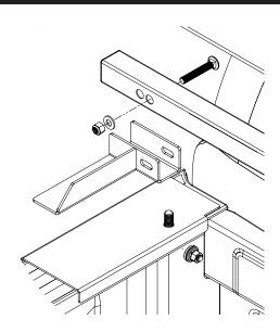
Fasten Backrack to the Rail mount bracket, or Toolbox bracket. Finger tighten at this stage.
