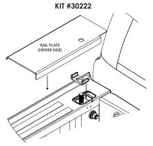
For the 30222 kit place rail plate over the stake pocket bolt and position notch against the front of the bed as shown
