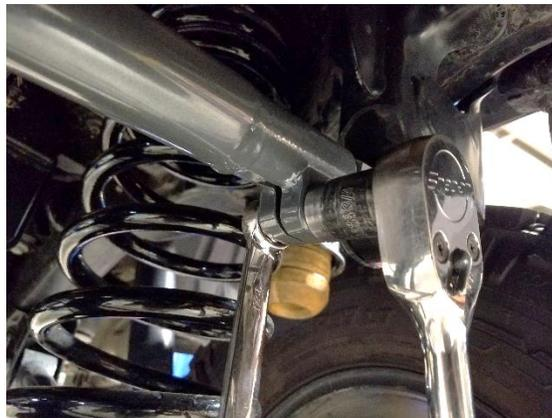
**Figure 7. Tightening the Pinch Bolt and Nut**
