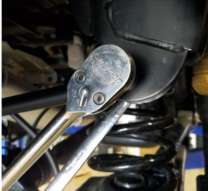
**Figure 2. Removing the Track Bar from the Frame Side**
