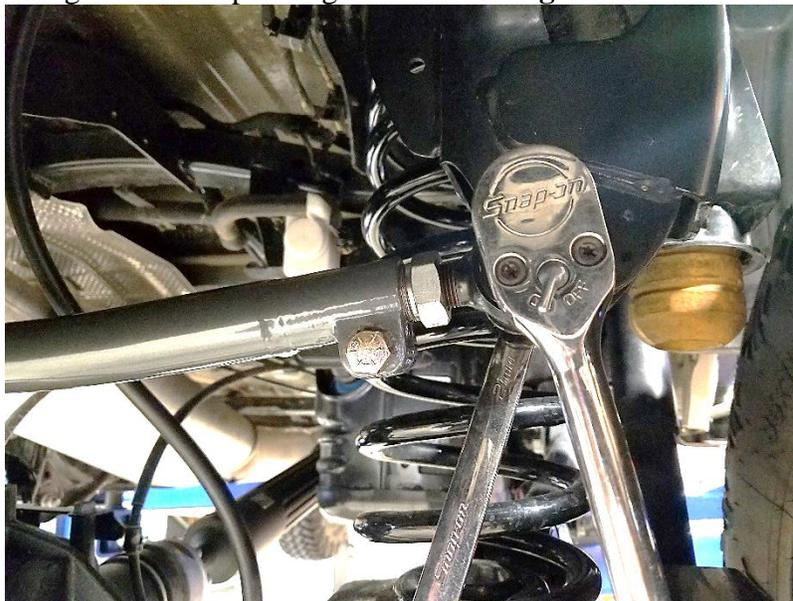
**Figure 3. Installing the Synergy Mfg. Track Bar at the Frame**
