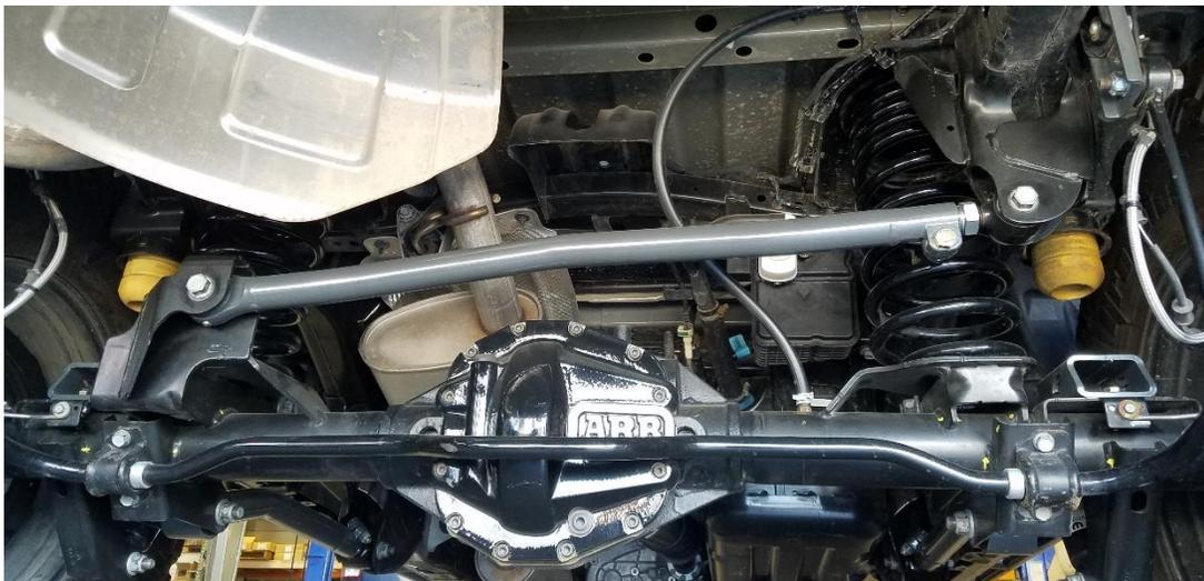
**Figure 5. Correctly Installed Synergy Mfg. Rear Track Bar**
