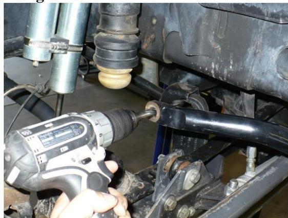
**Figure 1. Drilling Out the Sway Bar**
