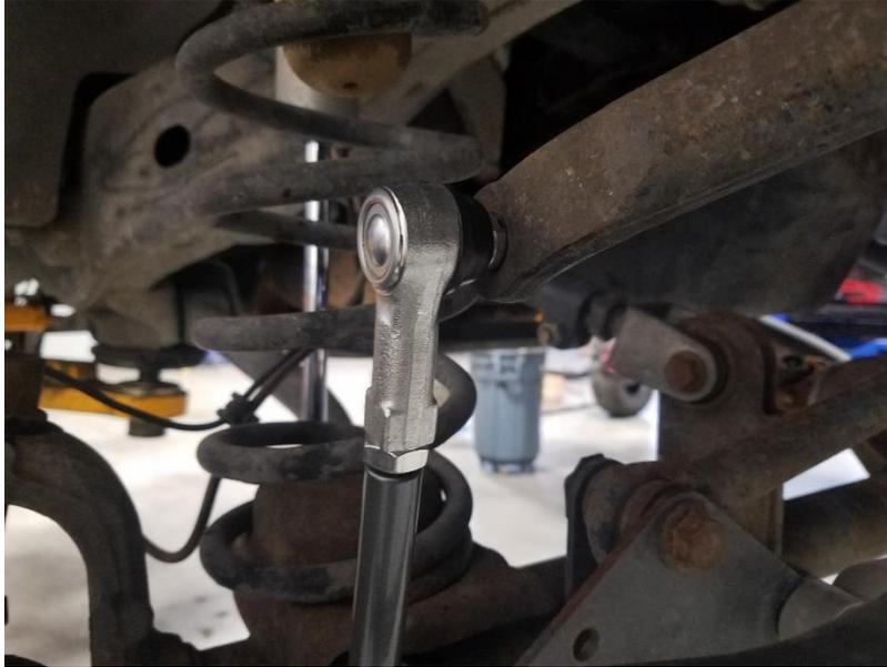
**Figure 2. Correct sway bar link rod end orientation.**
