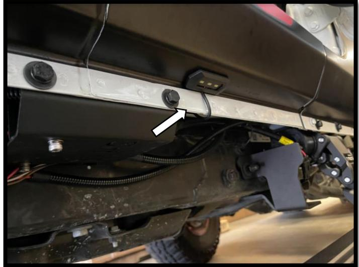
**Step 15:** Align the arrows on the small round connectors and plug the Passenger side front and Passenger side rear LED lights. Prepare the surface by cleaning with a 50/50 mix of isopropyl alcohol and water or equivalent. Once the surface is completely dry, peel the backing from the double-sided tape and stick the LEDs to the bottom side of the rocker panel. Position the LED lights at the center of the front and rear passenger side doors
