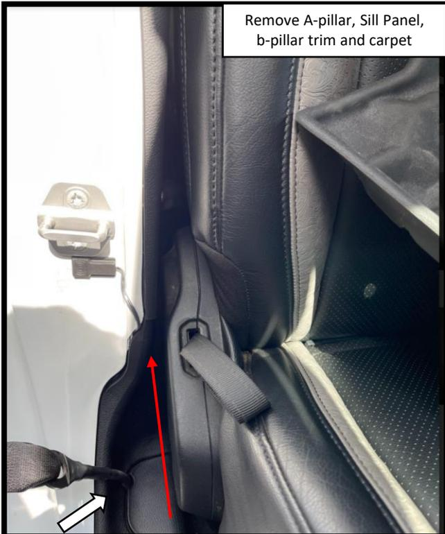
**Step 19:** Route the passenger side door trigger wire (brown) towards the passenger side b-pillar. Route the driver side door trigger wire (white) and the black disable switch wires under the center console to the left side of the vehicle. The white wire needs to go to the driver side b-pillar, the black wires will go to the center console.
