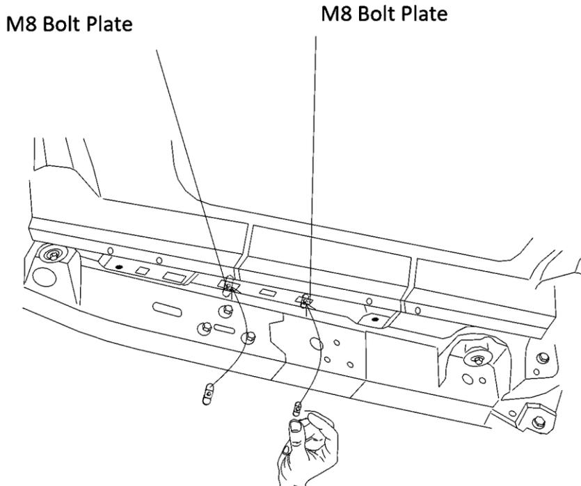
**Step 8:** Locate the paired square holes in the center of the body and insert the M8 bolt plates inside.
