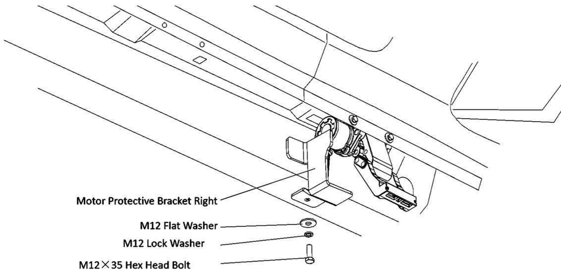
**Step 7:** Install the passenger side front motor protective bracket. Secure the protective bracket using an M12 hex bolt, flat washer, and lock washer. Torque to 25 ft-lbs.
