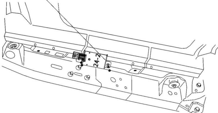
**Step 9:** Using two M8 hex head bolts, M8 flat washers and M8 lock washers, install the controller mounting bracket. Using a torque wrench, tighten to 18 ft-lb
