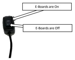
**Step 23:** Open the Driver side door and keep the door open. Flip the disable switch to the Off position. This will signal the running boards to retract to the stowed position and it will disable any further operation until the switch is flipped to the On position.
