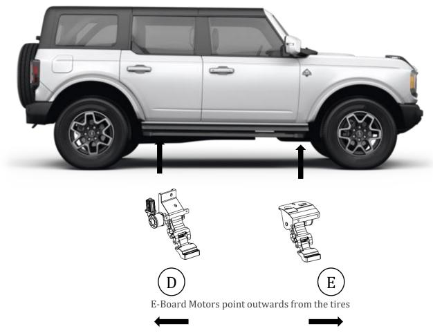
**Step 8**: Repeat Steps 1-4 to install the motor linkage assemblies on the passenger side. Repeat steps 6-7 to install running board on the Passenger side.
