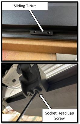
**Step 6**: Install the driver side running board. With assistance, begin by positioning the board on the front and rear motor assembly bases. Align the sliding T-Nut on the running board with the slots on the front and rear motor base. Once the T-Nuts are aligned, rotate the running board so that the T-Nuts set in the slots on the base of the arms. Repeat Steps 3-6 to install the motor linkage assemblies and running board on the Driver side.
