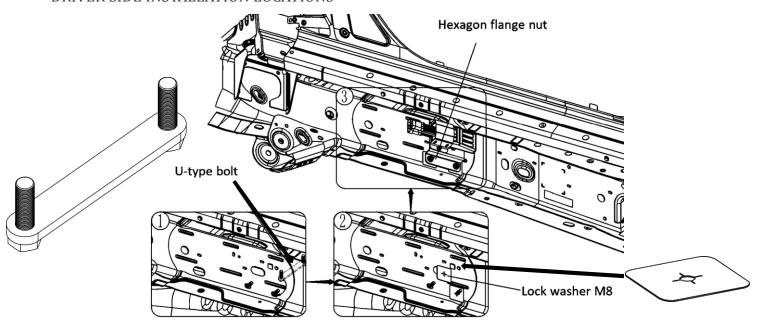
**Step 5**: Locate the hole near the center of the cab on the Driver side frame of the vehicle. Insert the bolt plate into the elongated hole and secure it using the M8 lock washer. Position the control module against the bolt plate and secure using (2) M8 Flange nuts.
