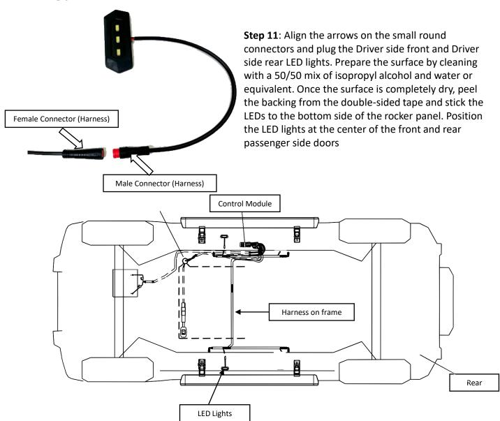
**Step 12**: Route the motor and LED wire harness from the controller to the Passenger side frame rail of the vehicle. When routing the harness keep clear from any moving parts and avoid direct contact with the exhaust system.
