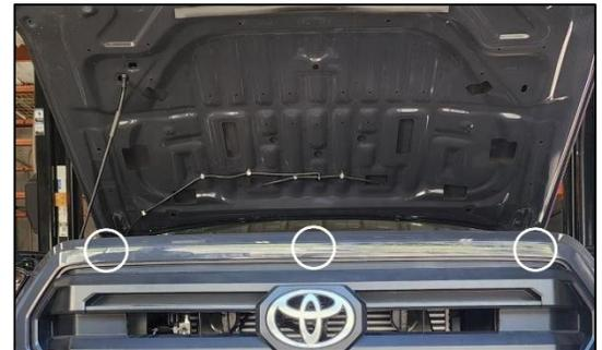
5. Remove the 6 bolts holding the shutter system in using a 10mm socket (circled). Use a Phillips head screwdriver to remove the small screws securing the front fog light cover. Stand the front clip up and remove the fog light cover starting at one end and disengaging the clips moving across.
