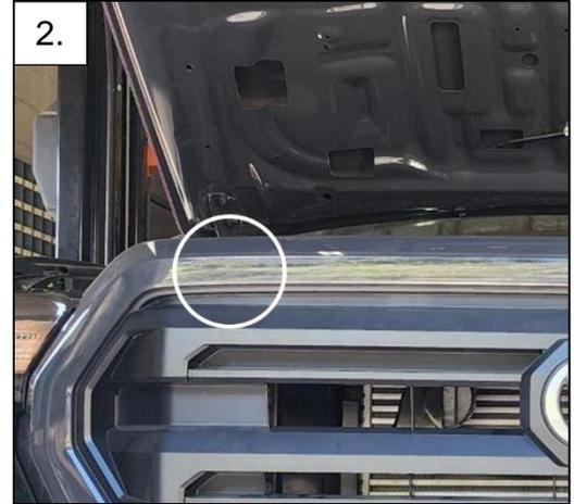
3. Gently pull the sides of the front clip out and forward to disconnect them from the vehicle. The furthest in clip will be behind the grill vent trim pieces. Repeat on the opposite side of the vehicle.
