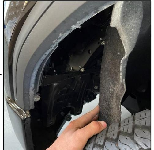
2. Using a 7mm socket, remove the 3x fasteners securing the fog light. Unplug the fog lights connector.
