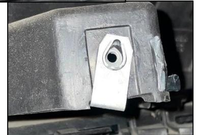
4. Install the S1's into the bracket as shown.
