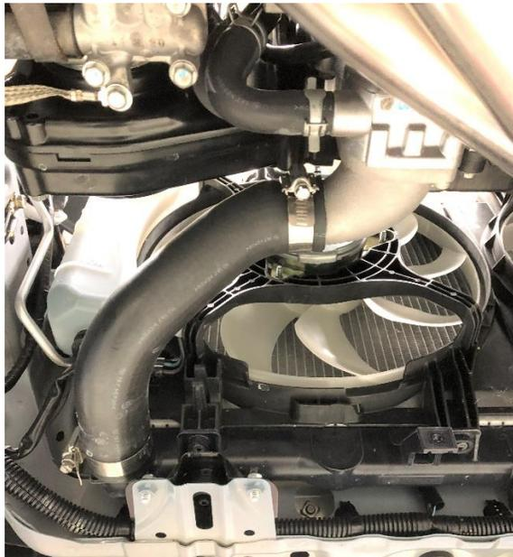
11. Once you have securely tightened the clamps and inlet, refill the coolant in the vehicle.
