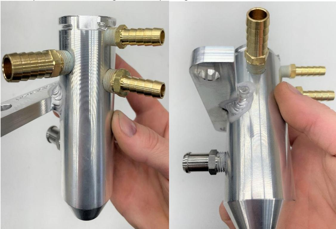
7. Use a socket wrench to tighten the (3) brass fittings.
