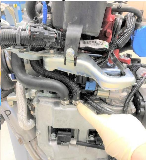
Perform this once on each rocker cover. Use a narrow flathead screwdriver to release the locking clamps: insert screwdriver in the gap on the side of the clamp, twist screwdriver to disengage clamps. Remove one 1/2" hose from each rocker cover port. Leave these hoses attached to the black breather pipe, which was fastened to the intercooler- leave it in place for future removal.
