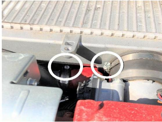
With a 12mm socket, socket wrench and extension, unfasten and remove the 3 bolts on the driver's side intercooler stay(bracket). Set aside for reinstallation.
