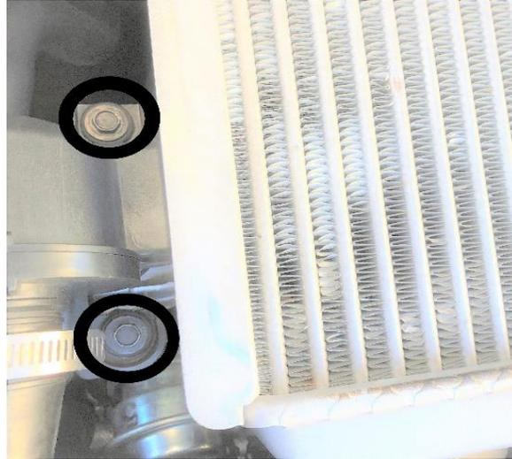
Remove the 12mm bolt that secures the intercooler to the passenger side intercooler stay(bracket).
