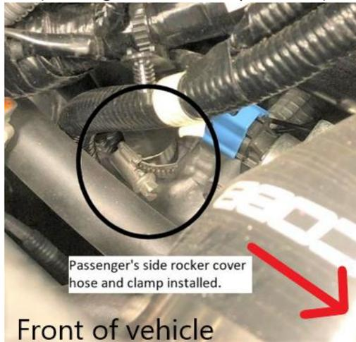
Install 3/4"x2.5" coupling hose on crankcase breather port. Orientate clamps so YOU can effectively tighten them. Tighten the clamp that secures the bottom of the tee in the 3/4"x2.5" coupling hose. The Tee, the drain hose and the 2.5" long section can be installed on the engine as one.
