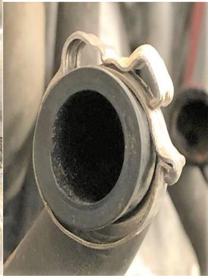
Remove one 1/2" clamp and hose from the smallest of the two rocker cover ports:
