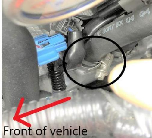
Install the 1/2"x28" RH rocker hose in the passenger side rocker cover port with a supplied hose clamp. (Passenger's side- front port=1/2")
