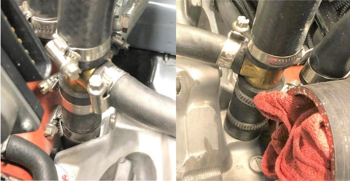
Install one end of the  $\frac{5}{8}$ "x24" hose on the fitting on the front of the turbocharger inlet, with a clamp. White connector is removed, clip transferred to engine harness grey connector and sealed off.
