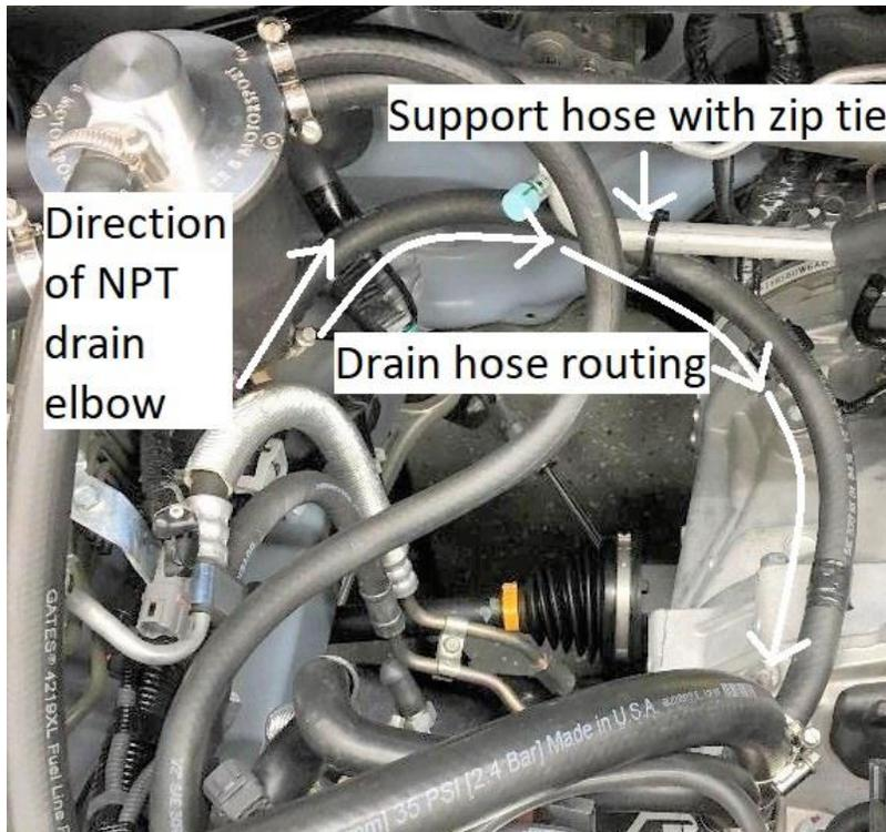
NOTE-This fitting is tapered- do not force the fitting to thread in beyond 60% of the fitting's thread length. The fitting should thread in approximately 3 revolutions before you need to use a wrench. Expect to see approximately 3-4 threads remaining once installed. The AOS may not drain effectively if the fitting is installed too deep/too tightly.
