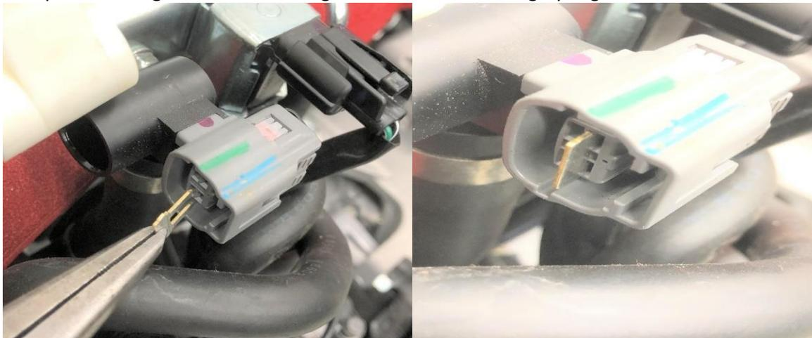
Using a small flathead screwdriver, release the tab and separate the hose fitting from the electrical connector and tape over the inlet of the connector to prevent liquid intrusion:
