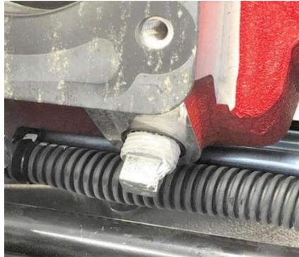
To remove the pcv assembly from the vehicle, locate the OEM  $\frac{3}{4}$ " diameter hose that the pcv connector is installed in. Loosen the clamp closest to the block (the clamp closest to the engine block, furthest down) by using a narrow flathead screwdriver: insert it into the gap in the side of the clamp and twist. With the clamp unlocked, twist the hose and pull up on the  $\frac{3}{4}$ " hose to remove it. Set aside for storage.
