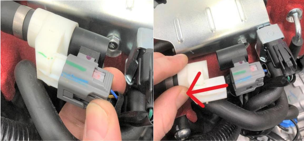
With needle nose pliers: pull metal shorting bar straight back while holding white connector:
