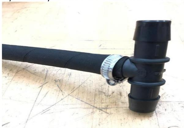
Install the 1/2"x39" LH rocker hose on the driver's side rocker cover port. Fasten the hose with a supplied clamp. (Drivers side- front port= 1/2")
