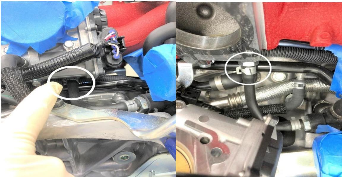
Using a 19mm deep well socket, remove the barbed fitting from the intake manifold. Set Aside for storage.
