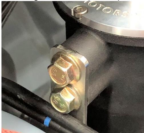
**The AOS should be perpendicular with the ground to effectively drain.**
