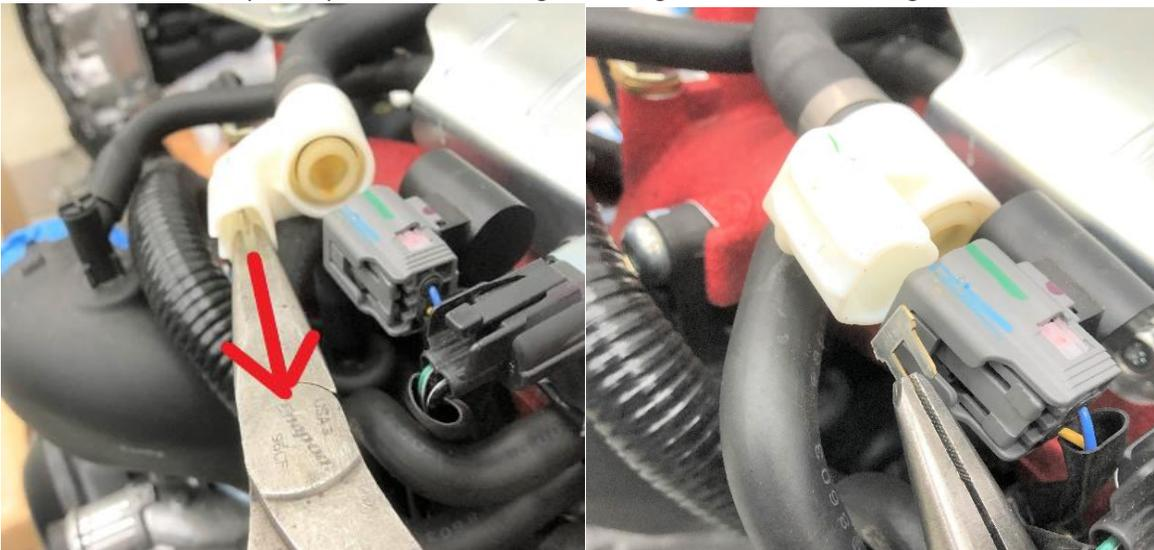
Flip the shorting bar around 180 degrees and insert it in the grey engine harness connector:
