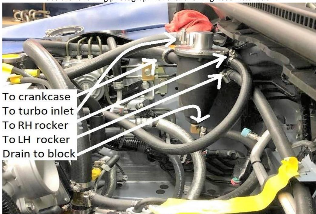
Take the unused end of the ½"x32" drain hose (the hose that intersects perpendicularly into the tee) and install it on the AOS drain fitting with a clamp. The hose should appear to route in a U-shape. You may secure it to an AC line with a zip tie, this will help prevent the hose from sagging and contacting the downpipe.
