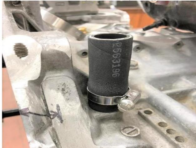
Once the hose is installed on the block and secured, insert the tee into the  $\frac{3}{4}$ "x2.5" hose and secure it with a clamp. Be sure to position the  $\frac{1}{2}$ "x32" drain hose so that it points back toward the firewall. This hose will soon be routed to the bottom of the AOS.
