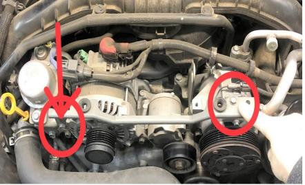
8. Remove the (2) push clips securing the airbox inlet duct to the upper radiator support. The airbox inlet duct can be set aside at this time.
