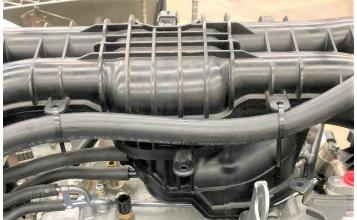
You may need to cut a small slot in the driver's side of your engine cover to allow clearance for the AOS suction hose.
