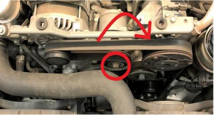
7. Loosen and remove the (2) 10mm headed bolts that secure the drivebelt cover bracket, set aside.
