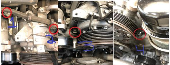
11. Take a pair of pliers and decompress the ½" hose clamp of the crankcase/coolant breather fitting, (the smaller fitting on the right side) Slide the clamp up so that you can take another set of pliers and loosen/remove the hose from the fitting.
