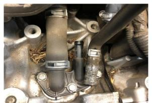
12. Locate the PCV valve and hose on the top of the engine. It is behind the intake manifold, on the passenger's side. Use pliers to loosen the hose clamp, slide it up the hose about an inch, lift the hose from the PCV valve. Remove the clamp. Grab the supplied hose plug and install it in the vacuum hose. Install the supplied SMALL zip tie to secure the plug in place. Tuck the plugged hose away so that it does not interfere with the remainder of this install.
