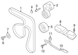
6. Place a 14mm wrench over the bolt on the front of the accessory drive belt tensioner. Rotate the wrench clockwise to decompress the tensioner, remove the belt. Set aside.
