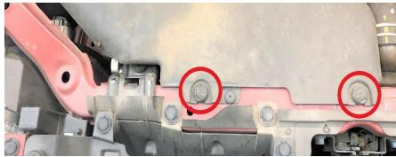
9. Unplug the passenger's side radiator fan and then loosen/remove the (2) 10mm headed bolts securing the fan to the radiator. Remove the fan from the vehicle. Set aside.
