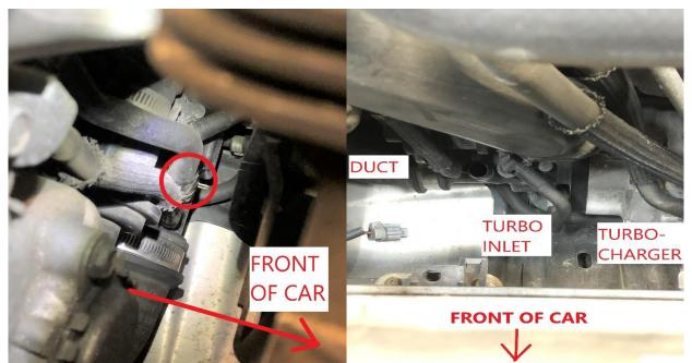
23. Grab the 5/8" x 52" long hose and install it where the factory tube was just removed from the turbo inlet, secure hose with a large hose clamp. Route the hose in the same path that the factory tube was. (Try to route the hose behind the charge pipe)
