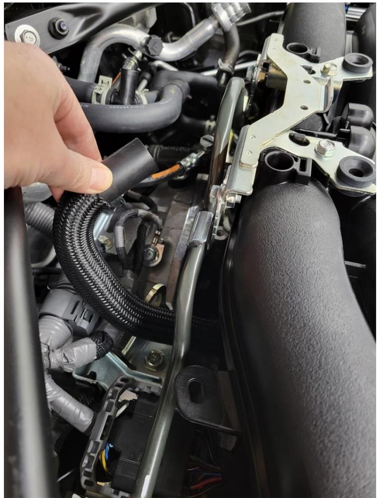
Step 7. Install Killer B Motorsport AOS with flanged ports. The hose on the Manifold port fits tightly. If you need to, use a drop of dish detergent or oil to help with install.
