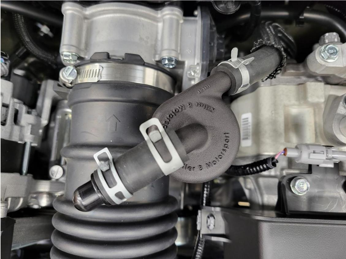
Step 6. Remove Rear PCV hose from Intake Manifold by twisting the PCV Valve hose ~45°
