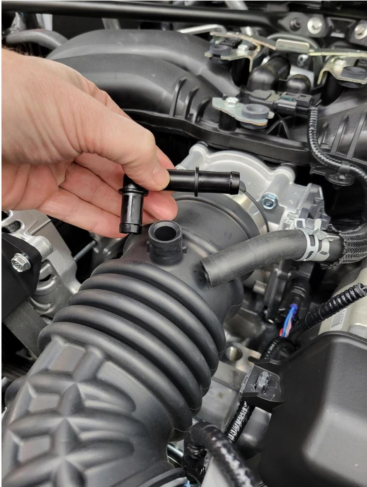
Step 3. Reverse Inlet Hose Elbow and reinstall OEM Hose Clamp
