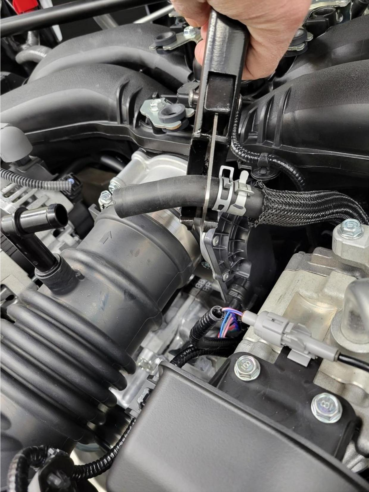
Step 5. Install Killer B Motorsport AOS with downward inlet port
