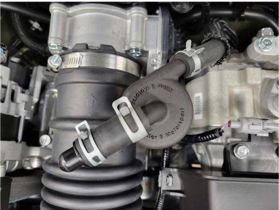
Step 6. Remove Rear PCV hose from Intake Manifold by twisting the PCV Valve hose  $^{\sim}45^{\circ}$
