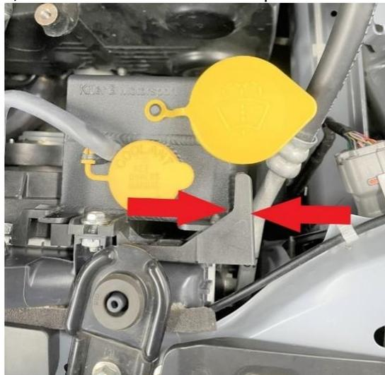
4. For 2018 and older models, skip to step 5. For 2019+ models, with the factory reservoir removed you will need to use a new hobby knife to trim the driver's side radiator fan shroud. (Remove a minimum of 1/8" of material from the areas marked in red)
