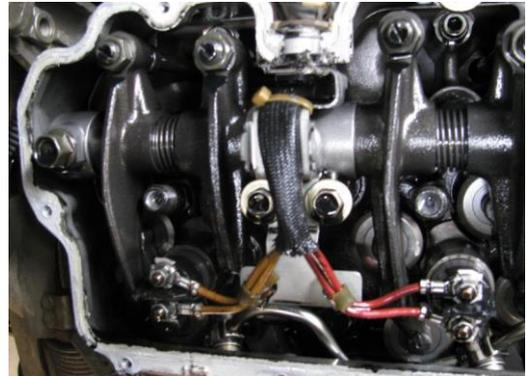
Remove 12 lower valve rocker arm cover bolts. Remove lower valve rocker arm cover. Remove gasket from lower valve rocker arm cover. Remove bolt grommets from lower valve rocker arm cover.
