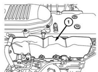
Remove fuel injector lines.
