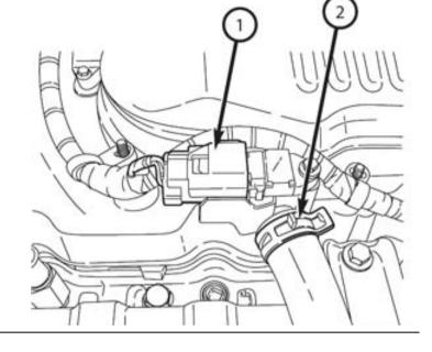
Remove the CCV oil drain hoses (1, 2) from cylinder head cover.
