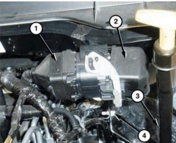
Cut cable tie and move aside the bulk head connector (1)
