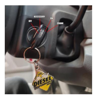
Crank engine. If the engine does not start after 25 seconds, turn key to OFF position, leave for at least 10 seconds. Repeat previous step until engine starts
