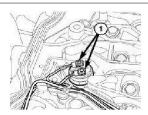
5. Reconnect both fuel injector harness connectors.
