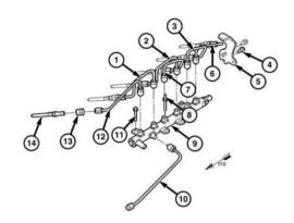
7.Remove the fuel injector connector nut.
