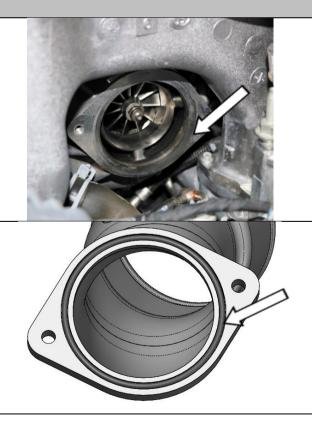
Place the turbo intake on to the turbo compressor-housing flange and secure it with supplied bolts as shown.
