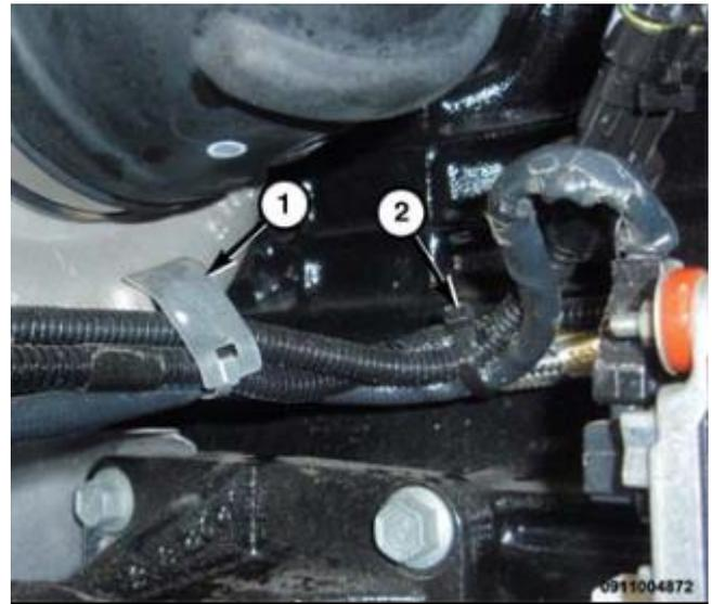
15. Remove bolt (2) and separate the retainer clip securing the wire harness and the turbocharger speed sensor wire harness to the turbocharger actuator.
